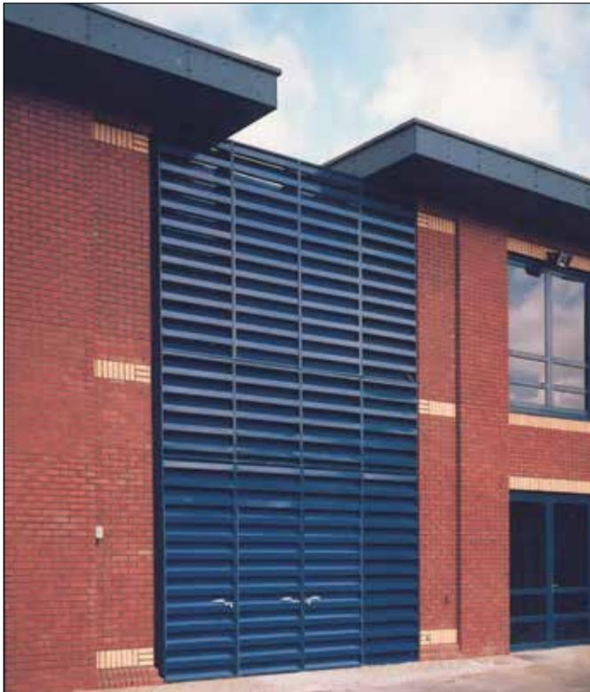
EMTEC LAAC 15 and LAAC 30 Acoustic Louvres can be installed as individual units or by bolting more than one unit together openings of any size can be accommodated. Each louvre has a robust outer framework which acts as vertical or horizontal mullions when several units are fixed together. If a continuous blade effect is preferred this can also be supplied.
